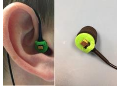
Figure 1. In-ear microphone holder for BRIR and HPIR measurements.
