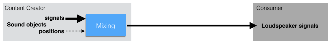
Figure 1. Channel-based Audio concept
